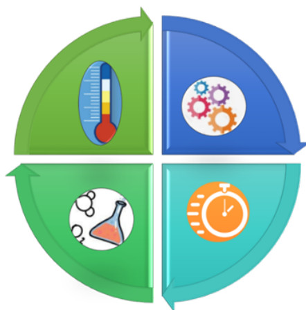
Fig. 1. Washing factors according to Sinner's cycle: time, temperature, mechanics and chemistry.
