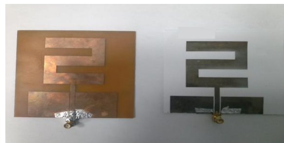
Figure 2: Figure illustrating Z-shaped antenna on glossy paper and PCB.
