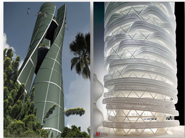
Figure 1. Architectural nanotechnology projects: NanoVentSkin (left) is a surface system that consists of nanoturbines that filter the air and produce energy and Carbon Tower (right) is made entirely out of carbon nanofibers.
